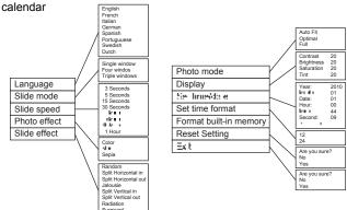
Select "SETUP" key to show setting menu,press "A/▼" key to select setting items,press ' ∢ / ▶ " key to adjust option,then press "ENTER" key to save the setting,press "MENU" key to return to the first-level menu,then press "MENU" key exit the setting menu.
